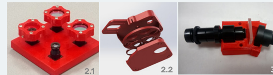
Figure 2: Low-cost multispectral cameras developed (CEBRA-M). Figure 2.1. Snapshot camera (left) Figure. Figure 2.2. Staring camera (right). Figure 3: Hyperspectral camera in Process of development (CEBRA-H.)
