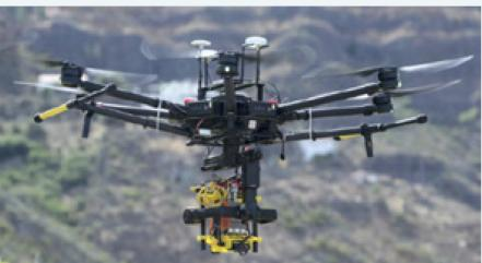
The present technology is a unmanned flying platform control system (drones) owning several different types of sensors (some of them multi -hyperspec- (• tral and RGB) that make possible to survey areas autonomously and recursively in order to provide real-time data about a specific surface.
