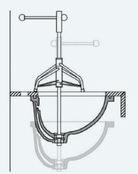
The designed device is able to support the weight of the washbasin or sink, allowing the installer to centre progressively the piece in the counter top cut-out as it fits to it without any corrections needed in the placement.
